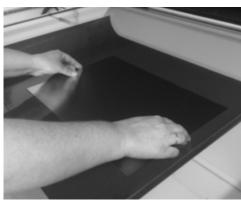
Carefully placing the photopolymer plate for the first exposure.
