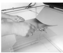
Placing the plate on the artwork for the 2nd exposure.
